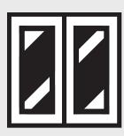
**Glazing:** 8 to 13.52 mm single glazing (toughened or laminated) in an overlapping or stepped arrangement.
