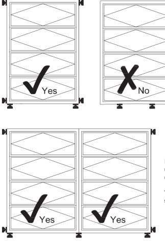
Packers must also be positioned under the centre mullion if applicable.
