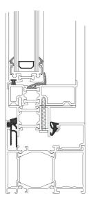
By using the appropriate adapter, all FIEGER louvre windows can be installed into existing window frames.
