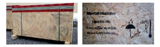
Packing crates should be offloaded using a fork-lift truck or similar device. After offloading, the crate & its contents must be checked for signs of damage and to ensure that the consignment is correct. In the event of any damage, missing or incorrect parts, FIEGER must be notified immediately and where possible, this must be noted on the delivery note.
