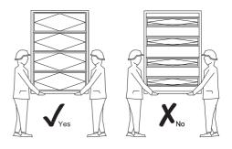
To prevent damage to the operating mechanism or glass breakage, the louvre window must be handled in a secure manner, i.e. no bending and twisting. Do not place or store on the corners.
