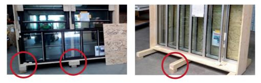
Prior to opening the crate, blocks should be used to lift the base of the crate. The box must be inclined slightly to the rear. This prevents the windows from falling out when the transport lock is released.
