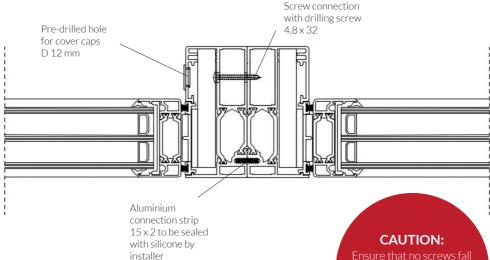
Ensure that no screws fall into frame during installation. This could block the operating mechanism!
