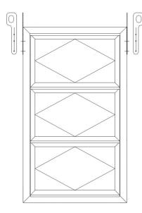
Screw size for fixing the Lifting Eyes: M6 x 20, Tightening torque 14 Nm
